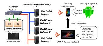
Figure 3: Configuration of demonstration.
