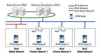
Figure 1: System configuration.
